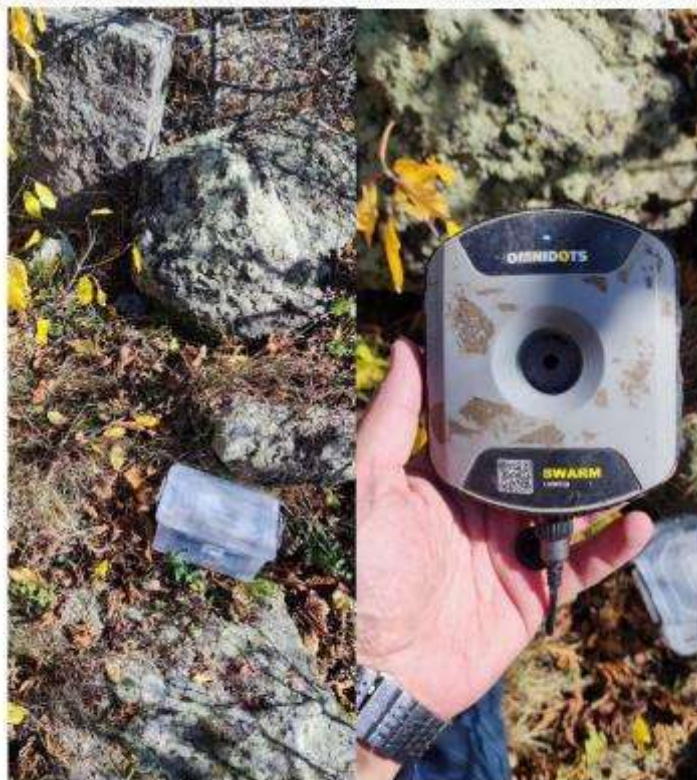
Figure 4.1: Vibration monitor SWARM was installed outside on the stone of the Monument
