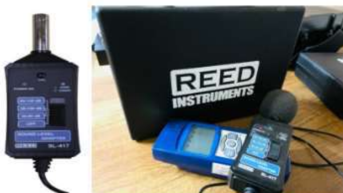
Figure 6.2.1 Noise level is determined by the REED INSTRUMENTS 9300 model adapter
