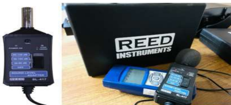
Figure 7.2.1 Noise level is determined by the REED INSTRUMENTS 9300 model adapter
